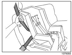
6) To tighten the belt, push down on the child restraint, pull the shoulder portion of the belt to tighten the lap portion of
